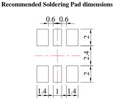
Unit: mm Tolerance: ±0.10mm
